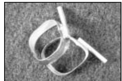
Extended tubes laser welded to band.
