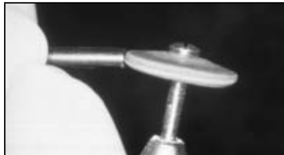
Edges smoothed with heatless stone or rubber wheel.
