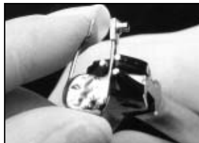
Correcting with 3-prong plier.
